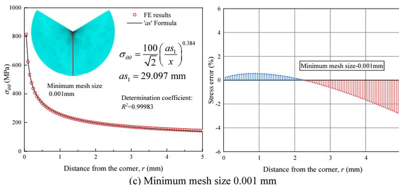
**Figure 5.** Stress errors between semi-analytic method and FE results with different mesh sizes
