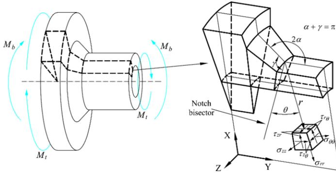
Figure 1. Polar reference coordinates system at a typical weld toe notch.
