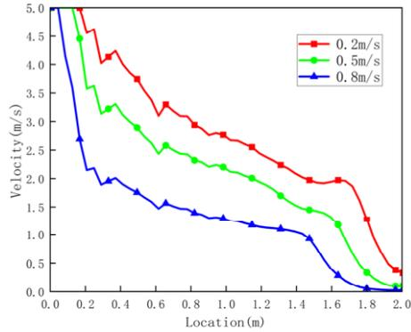
Figure 7. Variation of spray velocity along the axis of the outflow field at different liquid inlet velocities
