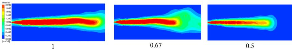
Figure 8. Spray velocity contour of outflow field under different gas-liquid channel diameter ratio
