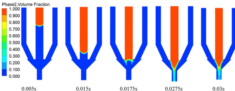
Figure 3. Gas-liquid two-phase distribution in axial section
