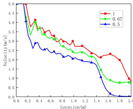
Figure 9. Variation of spray velocity in the outflow field along the axis under different gas-liquid channel diameter ratios
