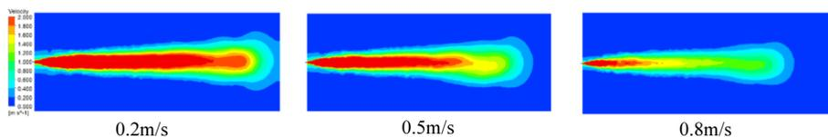
Figure 6. Spray velocity contour of outflow field under different liquid inlet velocity conditions
