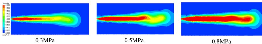
Figure 4. Spray velocity contour of outflow field under different gas pressure
