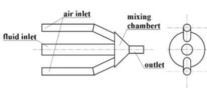
Figure1. Internal flow field calculation model of nozzle
