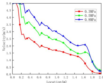
Figure 5. Variation of spray velocity along the axis of the outflow field under different gas pressure
