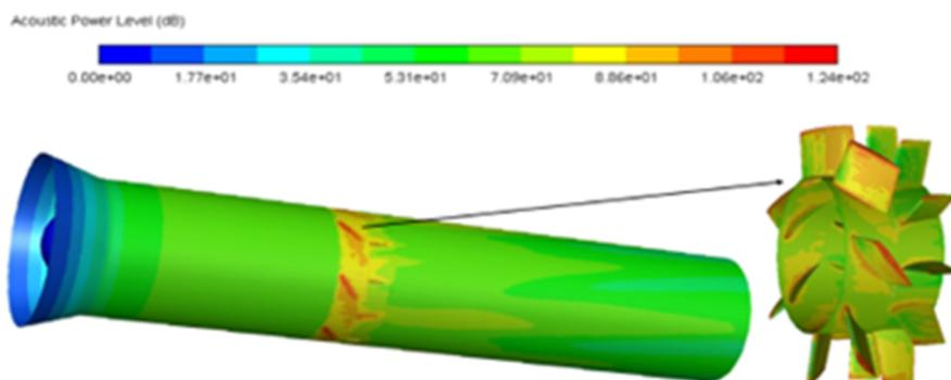
**Figure 5.** Cloud image of sound pressure level distribution of aerodynamic noise
