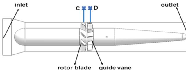
Figure 1. Mine axial fan structure schematic
