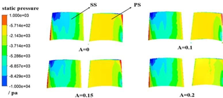
Figure 4. Comparison of static pressure cloud image of 4 kinds of fan blades
