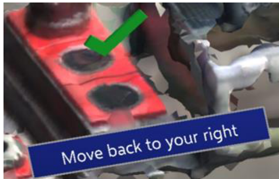
Figure 2. AR prototype: after a user performs a step correctly, a green checkmark appears, and the system moves to the next step.
