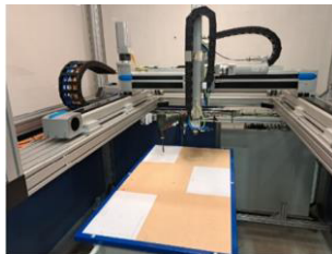
Figure 5. Gantry robot and a drill tool for verification of the place agent and coordinate transformations in skills. The three A4 sheets of paper on the table represent three pluggable process modules.
