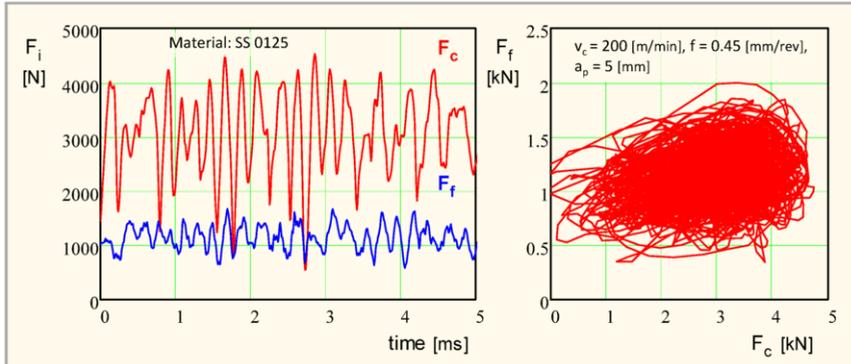
**Figure 8.** Examples of measured dynamic cutting forces, main cutting force  $F_c$  and feed force  $F_f$  during rough turning in gray cast iron SS 0125 (left) and corresponding load diagram (right).
