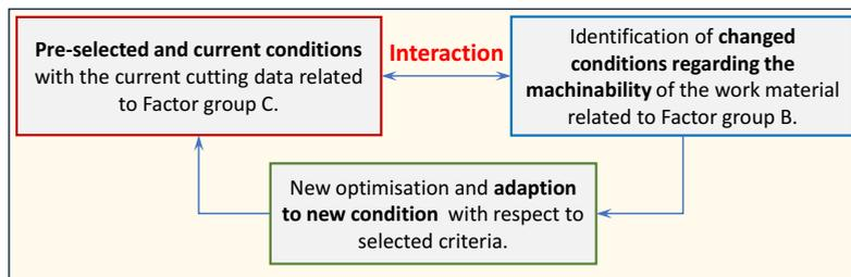
**Figure 5.** Adaptation and optimization of the machining process to changing conditions regarding the machinability of the work material.
