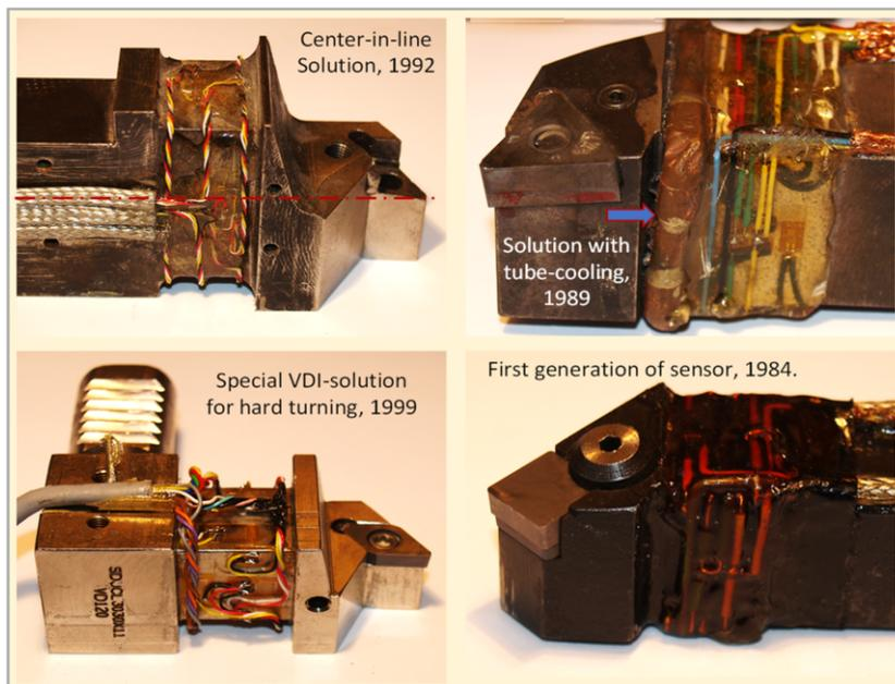
**Figure 9.** Example of a force sensor for measuring dynamic cutting forces with a relatively high bandwidth, developed at Lund University between 1984 to 1999.
