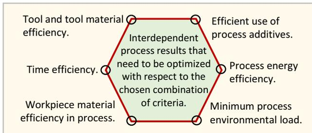
**Figure 3.** Performance and result parameters related to environmental load (ER), there the result parameters are depending on one or more factor groups related to machining.
