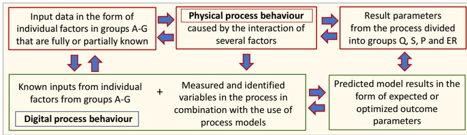
**Figure 4.** Relationship between factors and performance parameters (process outcomes) and how this can be optimized by measuring and identifying variables in the process that become input to process models.
