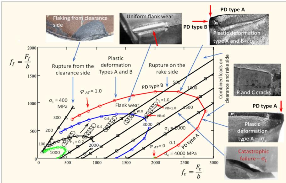
**Figure 7.** A schematic mechanical load diagram in which areas characterized by the occurrence of specific types of cutting tool degradation can be identified [4].
