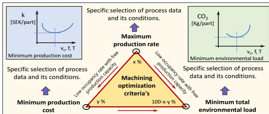
**Figure 2.** The balance or trade-off between the optimization criteria of maximum production rate, minimum production cost and minimum environmental impact.
