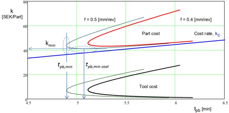
**Figure 1.** Example of a Hågglund cost and time graph where the part cost  $k$  and the tool cost are reported as a function of the production time  $t_p$  ( $t_{pb}$ ) for two different selected feeds  $f$  [9, 10].
