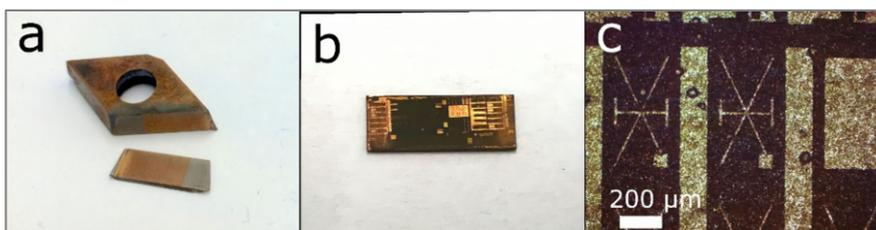
**Figure 11.** Example of a cutting tool that is sliced (a), a manufactured UV lithography pattern with sensor properties (b) and a magnification of a produced film-sensor (c).
