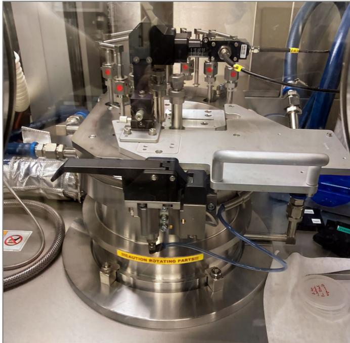
**Figure 10.** Research CVD-furnace used to produce different types of functional materials, including functional coatings that can be used for sensors.
