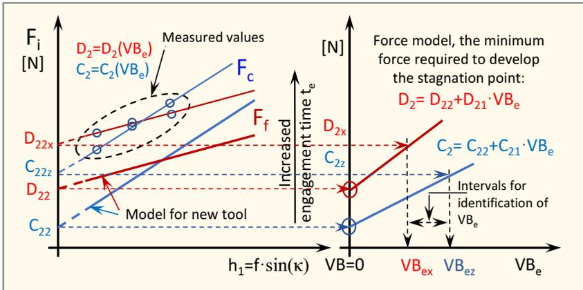
**Figure 6.** The principle of how an identification block is used, 6 or more measured values are recorded, by interpolation the constants (process variables)  $C_{2z}$  and  $D_{2x}$  are calculated (left) and by knowing the relationship between the process variables and equivalent flank wear  $VB_e$  can be estimated (right).
