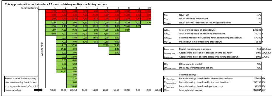
Figure 5. Screenshot of Excel file with data (12 months history) from the CMMS on the manual analysis of recurring failure on five manufacturing machines as well as approximations on cost of lost production time per hour, cost of spare parts per recurring failure as well as efficiency of the AI-model as well as the resulting maintenance actions.
