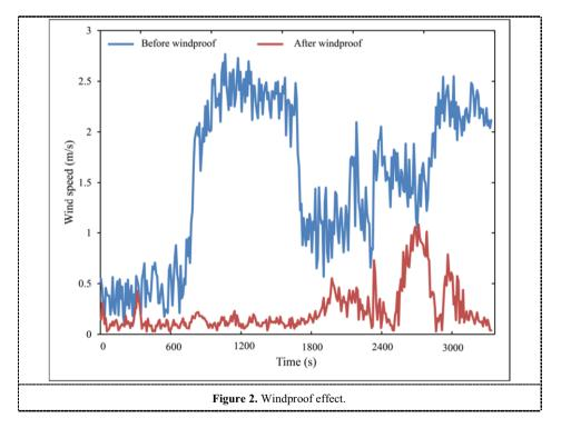
It can be seen from the test results that during the one-hour continuous test, when the environmental wind speed was below 3 m/s, the windproof module was able to reduce the environmental wind speed to below 1 m/s. When the environmental wind speed was less than 1 m/s, the impact of environmental wind on artificial snow production can be ignored. Therefore, the effect of environmental wind on snowfall simulation can be ignored in this snowfall simulation system.
