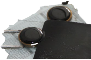
Figure 3. Scrape the softening point sample
