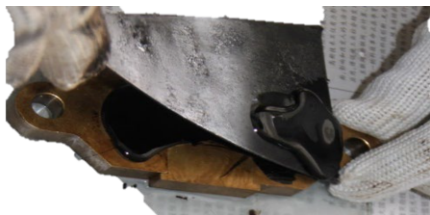
Figure 5. Scrape the ductility sample
