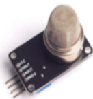
Figure 4. Smoke Concentration Detection Sensor
