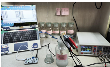
Figure 3. Saturated salt solution method testing process.
