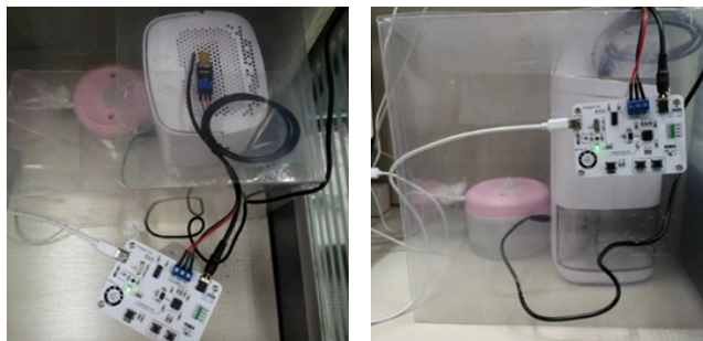
Figure 2. Constant Humidity Chamber Testing Environment.
