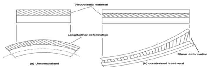
**Figure 5.** Basic viscoelastic damping arrangements
