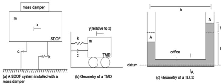
Figure 1. Modeling of an SDOF system and mass dampers
