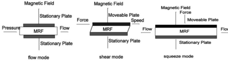
**Figure 7.** MR dampers under different operating conditions
