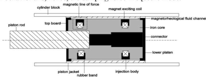
**Figure 8.** A sketch of the structure of the magnetorheological damper
