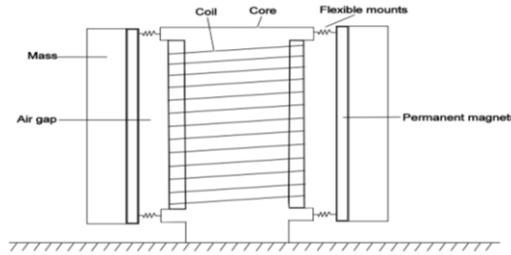
**Figure 6.** A sketch of the inertial actuator
