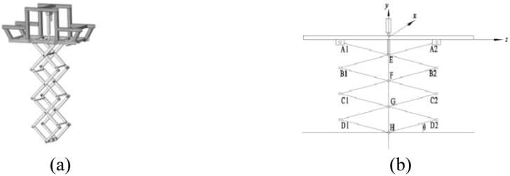
Figure 2. Charging bow end virtual prototype and mechanism schematic.
