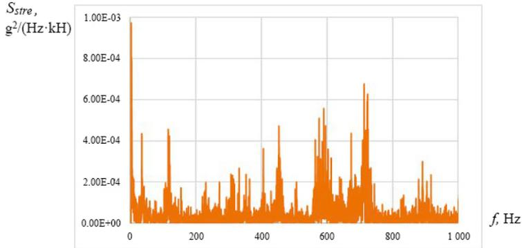
**Figure 1.** The reduced spectral density  $\bar{S}_{stre}$  of the vibration acceleration of the engine structure for the frequency range from 1 Hz to 1000 Hz
