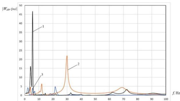
**Figure 2.** Dependences of the dynamic gain  $W_{str}(j\omega)$  of the rocket structure with the spacecraft (1 is single-staged LV with tandem layout, two is two-staged LV with tandem layout, 3 is LV with ‘core and strap-on boosters’ layout)
