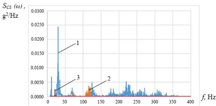
**Figure 3.** The calculated spectral power densities  $S_{cs}$  of vibration accelerations of the spacecraft structure for various launch vehicles (1 is single-staged LV of tandem layout, 2 is two-staged LV of tandem layout, 3 is LV of ‘core and strap-on boosters’ layout)
