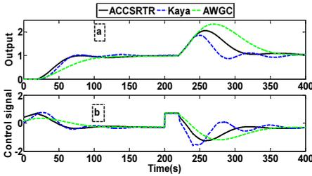
Figure 3. Nominal case results (a) Closed-loop system outputs, (b) Control efforts.
