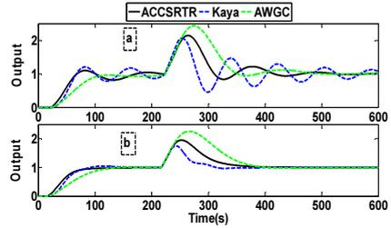
Figure 4. Closed-loop system outputs for variations in system parameters (a) +15%, (b) -15%
