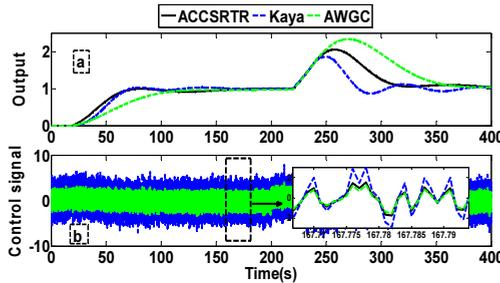
Figure 5. Closed-loop system outputs under measurement noise with a power of 0.0001 (a) Closed-loop system outputs, (b) Control efforts
