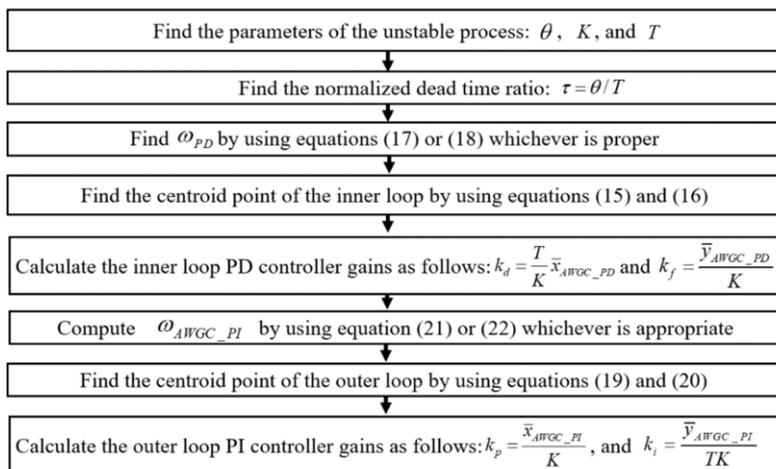
Figure 2. A flowchart for computing the parameters of the PI-PD controller using the proposed method
