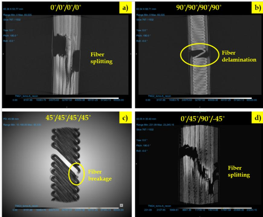
Figure 4. Micro CT images of fractured specimens
