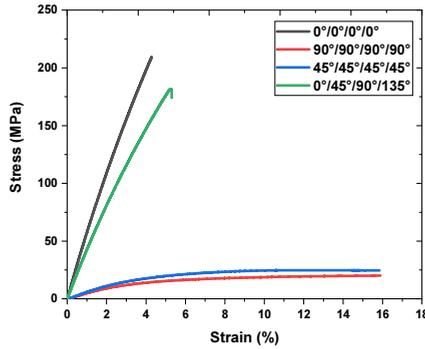
Figure 2. Stress strain curve for tensile strength
