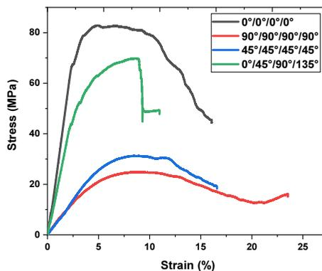
Figure 3. Stress strain curve for flexural strength
