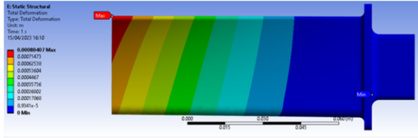
Figure 6 Deformation analysis without thermal load.
