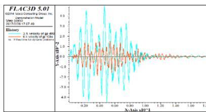
Figure 11. Time history diagram of x-direction velocity at monitoring points of bedrock and sliding mass after earthquake action.
