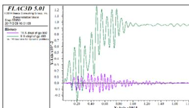
Figure 10. Time history diagram of displacement in the x-direction of monitoring points for bedrock and sliding mass after earthquake action.
