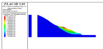
Figure 9. Schematic diagram of landslide displacement slice after earthquake action
