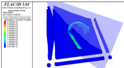
Figure 6. Distribution of shear strain increment and landslide mass after earthquake.
