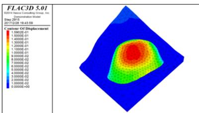
**Figure 3.** Distribution characteristics of landslide displacement under gravity field.
