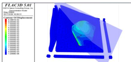
Figure 8. Shear strain increment distribution and slice position of landslide body after earthquake
