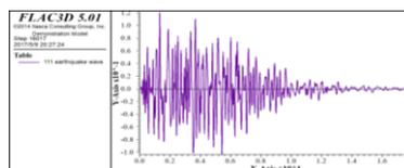
**Figure 5.** Input FLAC3D seismic wave acceleration the spectrum.
