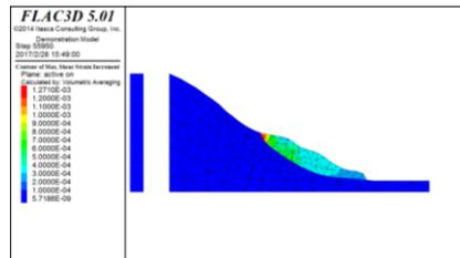
Figure 7. Schematic diagram of shear strain slice position of increment slice of landslide mass after earthquake.
