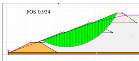
**Figure 13.** Upstream triple staged dyke model without proper drainage, downstream slope 2H: 1V and upstream slope 3H: 1V, using sample B.
