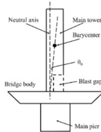
Figure 2. Simplified schematic diagram of the main tower.
