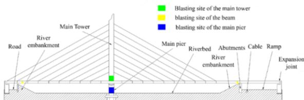
Figure 1. Schematic diagram of Jinwu Bridge structural model.
