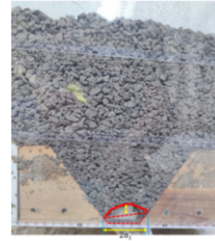
Figure 6. Pea stone trapdoor test arching diagram.
