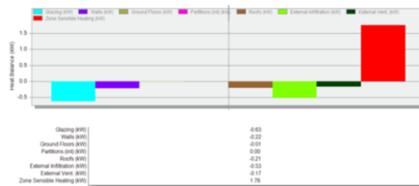
Figure 5. Heat Loss through the Envelope and Ventilation.
