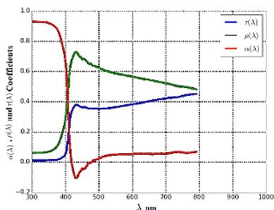
**Figure 2.** Spectral transmission, reflection and absorption coefficients of the sample "Acrylic 4mm WOP 35%"
