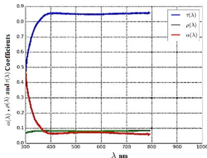
**Figure 7.** Spectral transmittance, reflection and absorption coefficients of the sample "Gpps polystyrene with 2mm crushed ice embossing" (light falls on a smooth edge).
