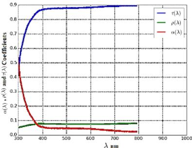
**Figure 6.** Spectral transmittance, reflection and absorption coefficients of the sample "Gpps polystyrene with 2mm crushed ice embossing" (light falls on the corrugated edge).
