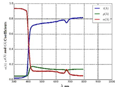
**Figure 4.** Spectral transmission, reflection and absorption coefficients of the sample "Monolithic polycarbonate 2mm diff 80%"
