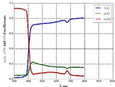
**Figure 5.** Spectral transmission, reflection and absorption coefficients of the sample "Monolithic polycarbonate 1.5mm diff 90%"
