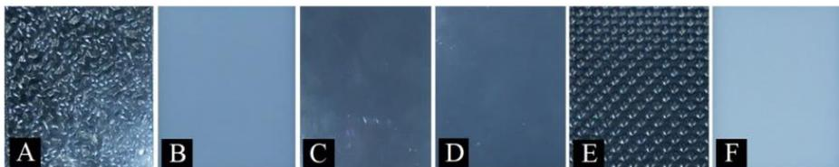
**Figure 1.** Samples prepared after hand lay-up molding process technique. (A)-Acrylic 4mm WOP 35%, (B)-Monolithic polycarbonate 1.5mm diff 60%, (C)-Monolithic polycarbonate 2mm diff 80%, (D)-Monolithic polycarbonate 1.5mm diff 90%, (E)-Polystyrene gpps with 2mm “chipped ice” embossing (light falls on the corrugated edge), (F)-Polystyrene gpps with 2mm “chipped ice” embossing (light falls on a smooth edge).
