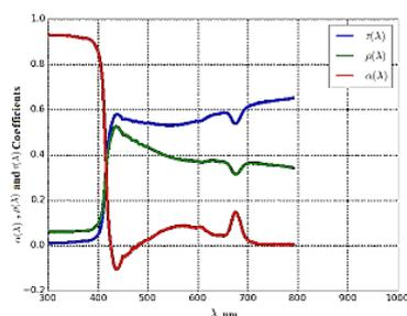
**Figure 3.** Spectral transmission, reflection and absorption coefficients of the sample "Monolithic polycarbonate 1.5mm diff 60%"
