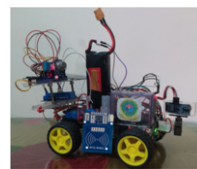
Figure 13. Prototype Version of IoT-Driven Sophisticated Robot leveraging RFID Identification.
