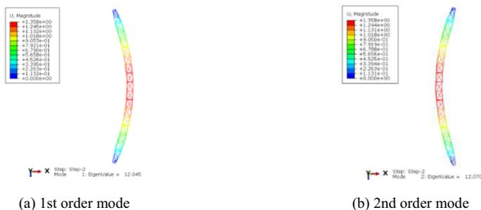
Figure 12. The first two order buckling modes of leg.
