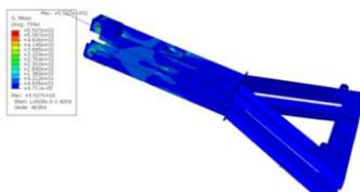
**Figure 6.** The stress of pulley bracket.
