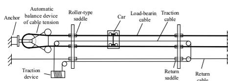
**Figure 3.** The diagram of continuous-double-cable freight ropeway (top view).
