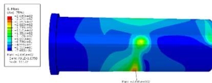
Figure 10. The stress of wheel axle.
