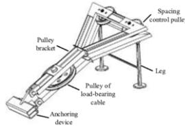
**Figure 4.** The automatic balance device of cable tension.
