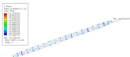
Figure 11. The stress of support leg.
