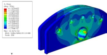
Figure 8. The stress of roller plate.
