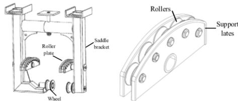
**Figure 5.** The diagram of roller-type saddle.
