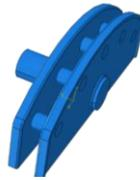
Figure 7. Finite element model of roller-type saddle.
