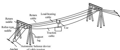
**Figure 2.** The diagram of continuous-double-cable freight ropeway.
