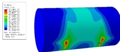
Figure 9. The stress of roller axle.
