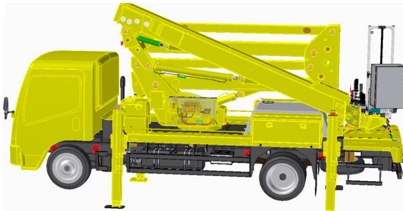
Figure 2. Virtual prototype model of pillar insulator string cleaning robot.
