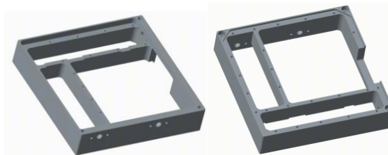
Figure 1. Three-dimensional model of the upper and lower ends of the shielding box
