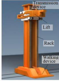
Figure 1. Basic Structure of Lifting Jack.
