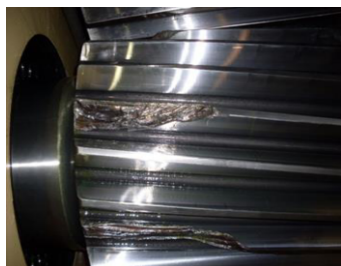
Figure 1. Fracture diagram of teeth root.
