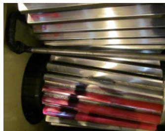
Figure 2. Gear sub contact spot diagram.
