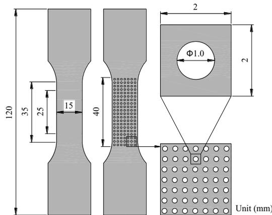
Figure 1. Grid shape and reference point marking for measurement of displacement.
