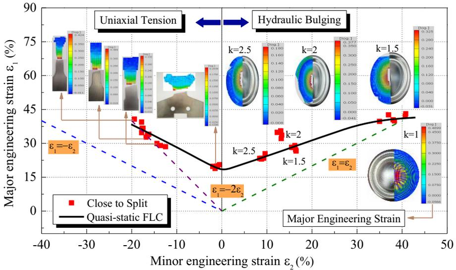
Figure 4. Experimental FLD of DP600 steel sheets.
