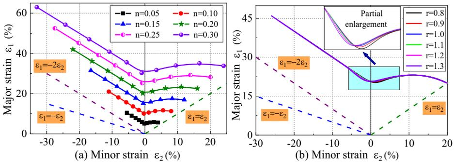
Figure 6. Theoretical prediction by Hill'79 yield criterion with various (a)  $n$ -value and (b)  $r$ -value.
