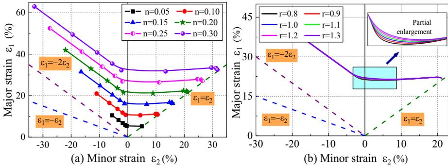
Figure 7. Theoretical prediction by Logan-Hosford yield criterion with various (a)  $n$ -value and (b)  $r$ -value.
