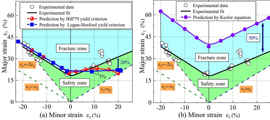
Figure 5. Comparison of experimental data to theoretical FLCs: (a) various yield criteria, (b) Keeler equation.
