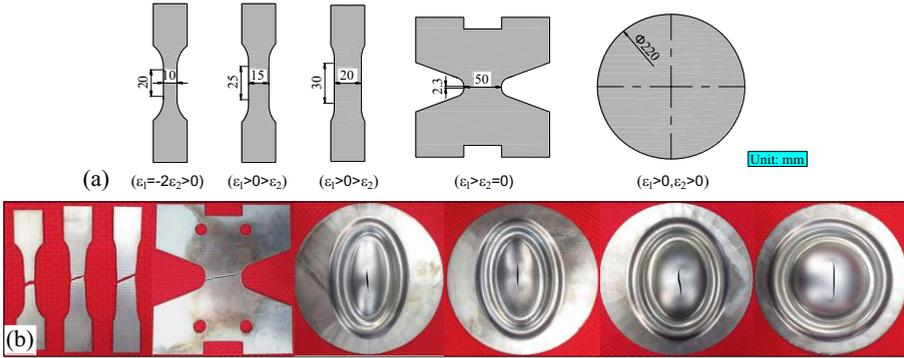
Figure 3. Initial specimen geometries (a) and fractured specimens (b) under different strain paths.
