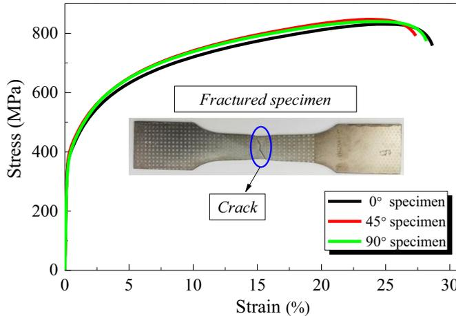
**Figure 2.** The fracture specimen and stress-strain curves of DP600 steel sheets.
