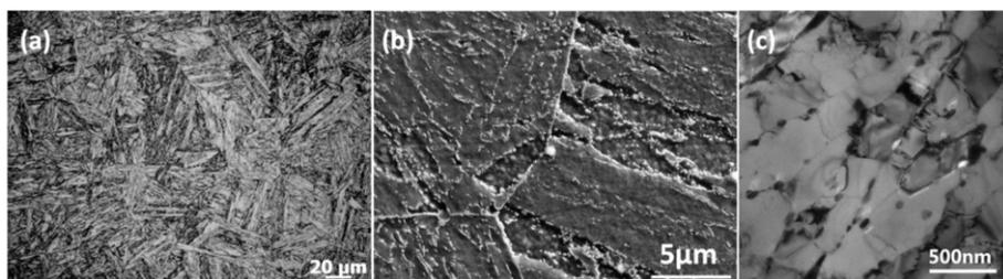
**Figure 1.** The initial microstructure of G115 steel: (a) OM; (b) SEM; (c) TEM.
