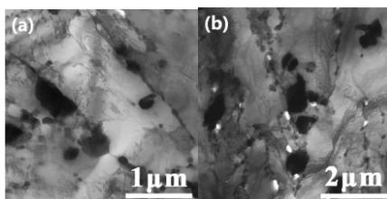
**Figure 3.** TEM micrographs of the studied steel aged at (a) 650°C and (b) 700°C for 8000 hours.
