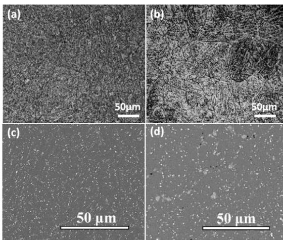
**Figure 2.** The microstructure of G115 steel after thermal exposure at (a) and (c) 650°C; (b) and (d) 700°C for 8000 hours: (a) and (b) OM mode, (c) and (d) BSE mode.
