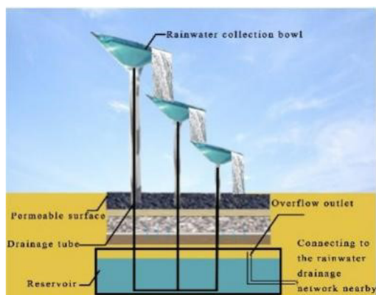
Figure 2. Sectional drawing of infiltration and circulation facility.
