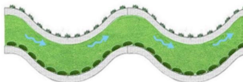
Figure 4. Schematic diagram of the curved grassed swale.
