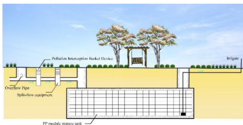
Figure 6. Landscape design drawing of the modular storage tank.
