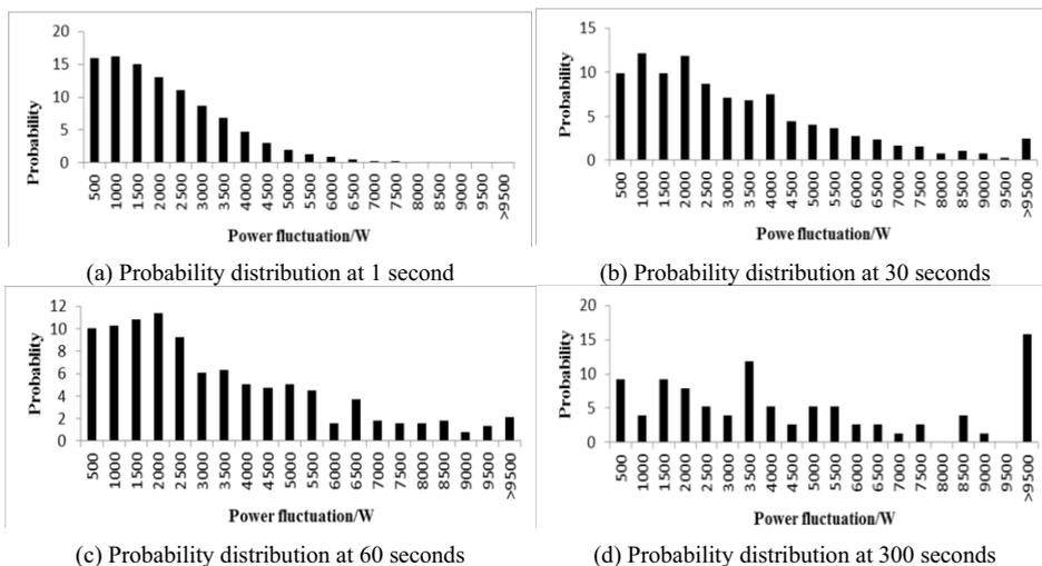
Figure 7. Probability distribution of power fluctuation at different sampling intervals.
