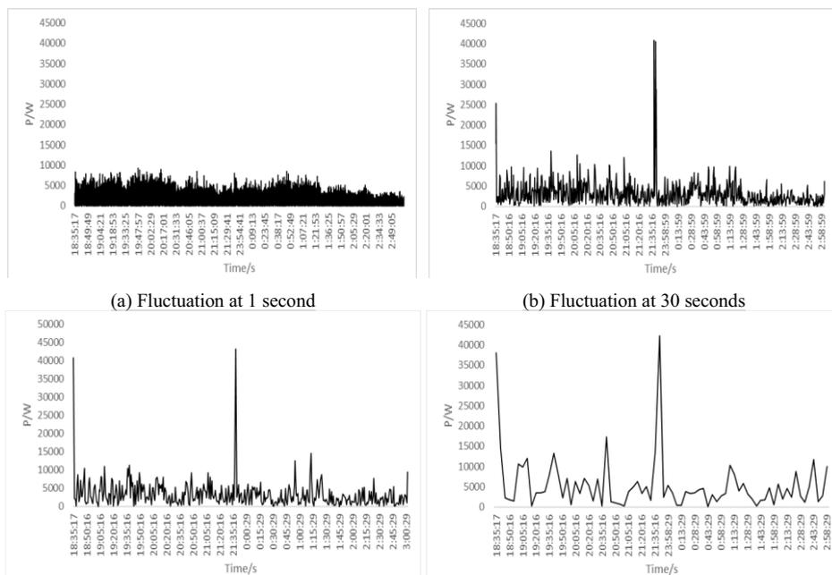
Figure 6. Variation of power fluctuation with sampling interval.
