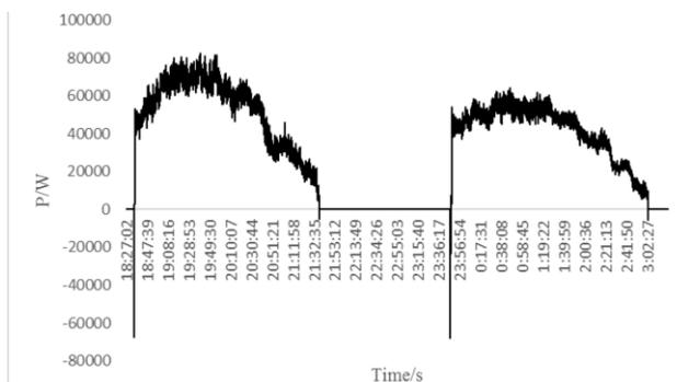
Figure 1. Real-time power of rising and falling tide.
