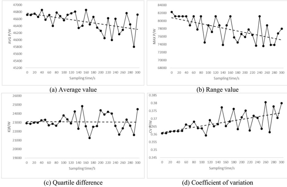
Figure 2. Relationship between the discrete index and sampling interval.
