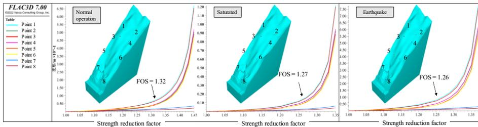
Figure 3. FOS of the slope under three different operation cases.
