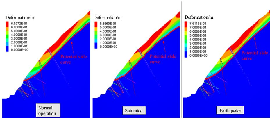
Figure 5. The deformation of 0+152 m cut of the slope in different operation cases.
