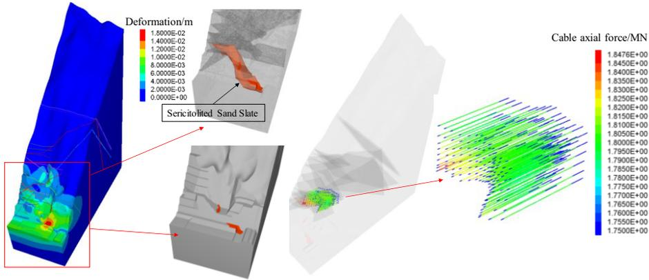
Figure 2. Slope deformation and cable stress after excavation and support.
