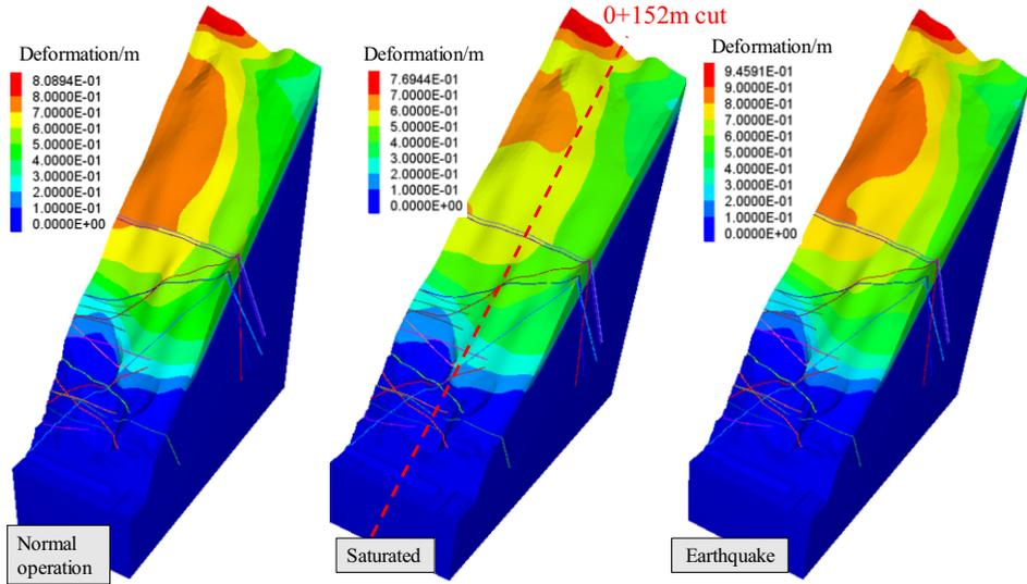
Figure 4. The deformation of the overall slope in different operation cases.
