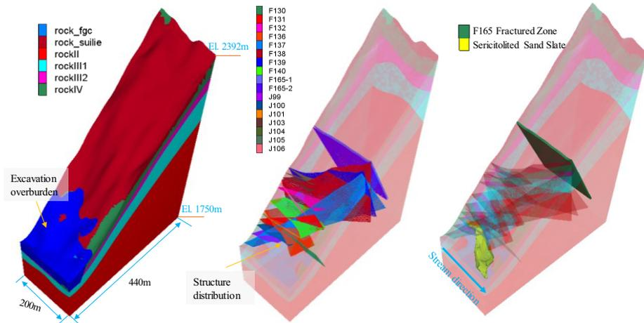
Figure 1. Numerical model of the slope and structures in FLAC<sup>3D</sup>.
