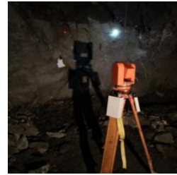
Figure 4. Automatic cross-sectional measurement
