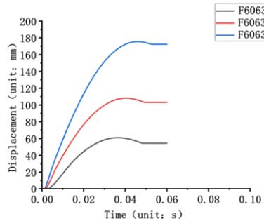
Figure 11. F6063 Impact data diagram.
