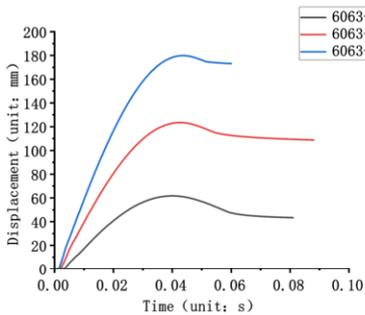
Figure 10. 6063 Impact data diagram.
