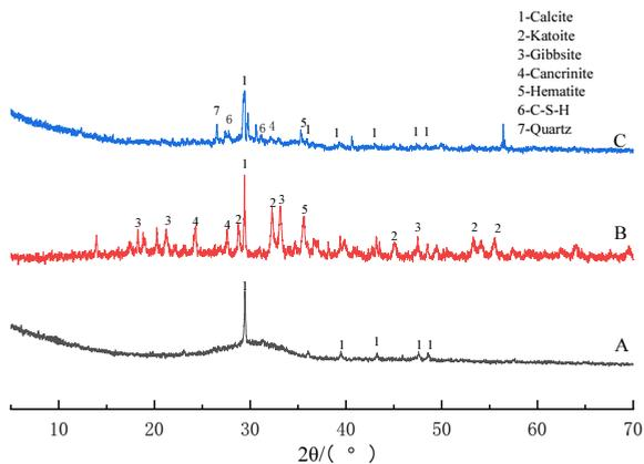
Figure 5. XRD diffractogram (A - mineral powder, B - red mud, C - ZJ-9)
