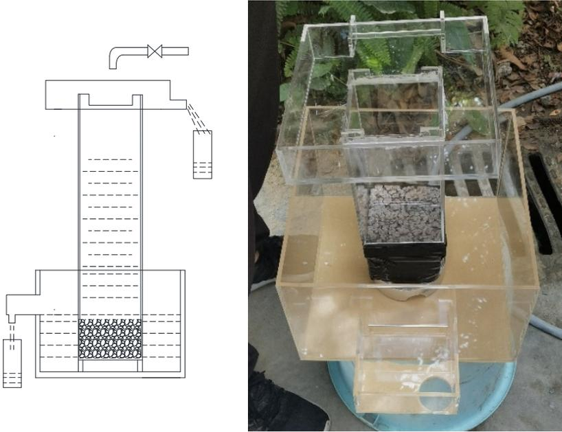
**Figure 1.** Home-made water permeability tester
