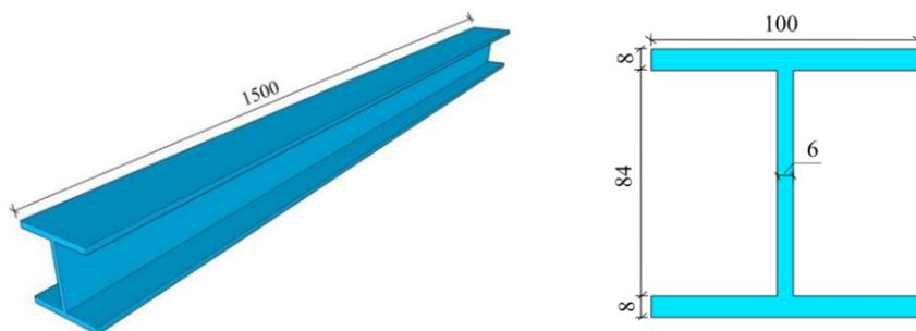
**Figure 2.** Structural Drawing of H-shaped Steel Structure
