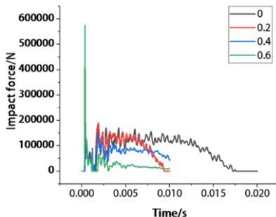
**Figure 5.** Time history curves of impact force under different axial loads
