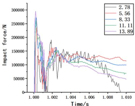
Figure 6. Time history curve of impact force at different speeds
