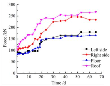
**Figure 12.** Typical monitoring curves of high-strength hollow grouting anchor cables
