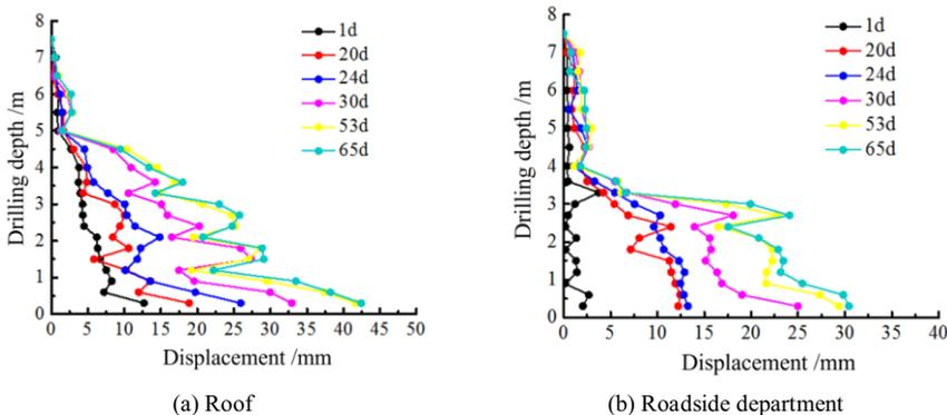
Figure 10. Typical monitoring curves of roadway internal displacement
