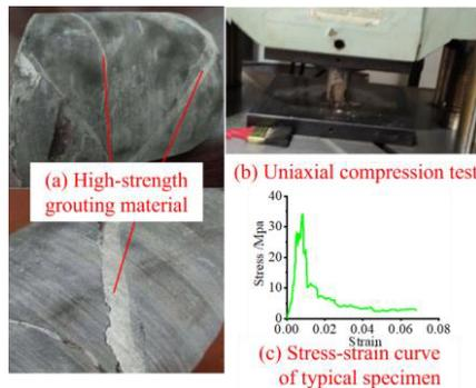
**Figure 8.** Core-drilling of rock mass after grouting and laboratory test
