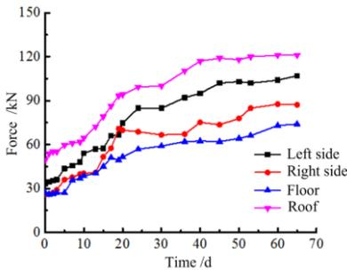
**Figure 11.** Typical monitoring curves of high-strength grouting bolts
