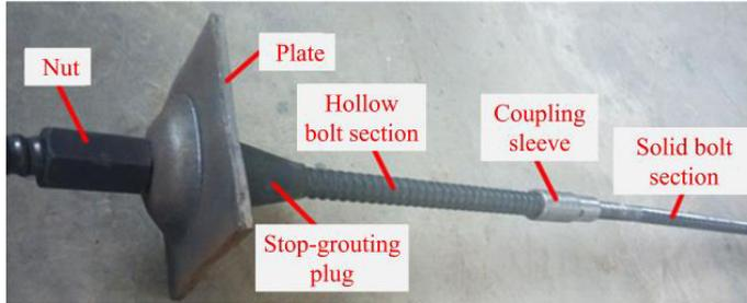
Figure 5. Combined high-strength grouting bolt
