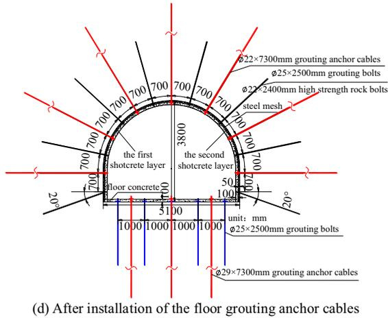
**Figure 7.** Cross-sectional design drawing of high-strength bolt-grouting support under different stages
