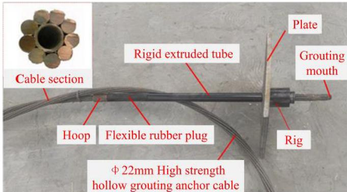
Figure 6. High-strength hollow grouting anchor cable
