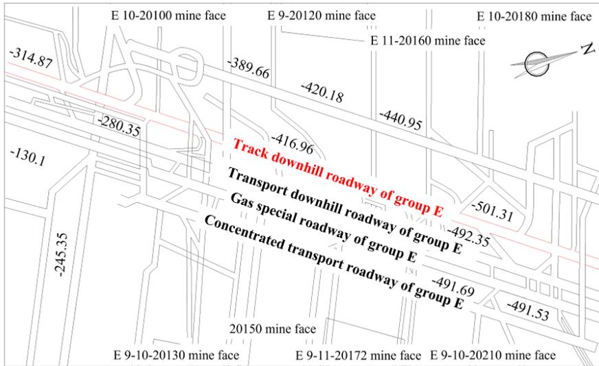
**Figure 2.** Layout plan of downhill roadways of group E in central area
