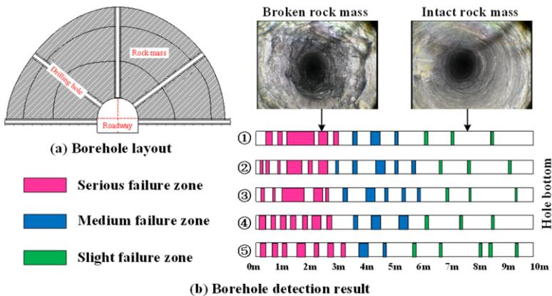
Figure 4. Detection results of failure range of rock mass in field roadway
