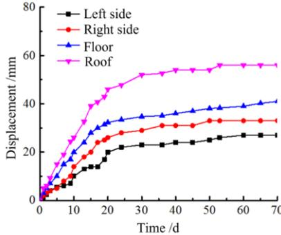
Figure 9. Typical monitoring curves of roadway surface convergence displacement
