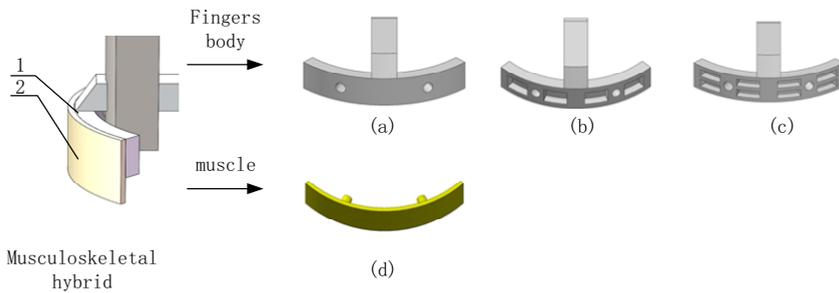
1. Finger body: (a) surface with round hole; (b) surface with round holes and 4 large square holes; (c) surface with round holes and 8 small square holes. 2. Finger muscle
