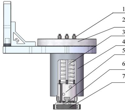
1. Guide rod 2. Connecting plate 3. Spring 4. Cylinder 5. Tubular palm 6. Finger body 7. Fingerpad
