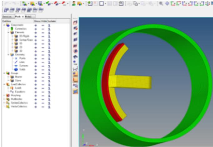
**Figure 4.** The finite element model of the finger impacting fragile parts
