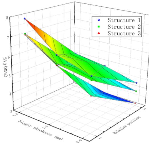
**Figure 6.** The relationship between finger structure and parameter to the maximum contact stress in grasping contact collision
