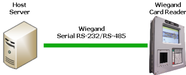
Figure 4. A typical Card-based Access Control System for vehicles in Truck-Loading Fuels Terminals.
