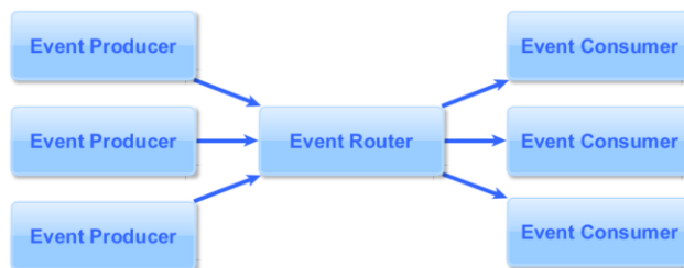
Figure 3. IoT Event-Driven Architecture.
