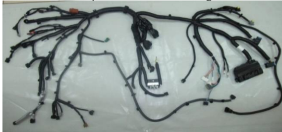
Figure 1. Example of Electrical Engine Harness
