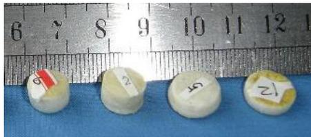
Figure 3. The implants fabricated by 3D printing.
