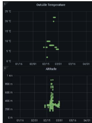
Figure 2. Evolution of outside temperature and altitude for BMW 116d during preliminary tests.
