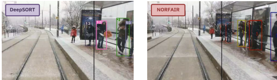
(b) Station 2 (Snow): The actual number of passengers is 7, our system using the Tracking Algorithm with DeepSORT predicted 8 people (left), while with the NORFAIR predicted 8 people (right).
