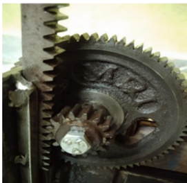
Figure10: Rack and pinion arrangement
