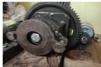
Figure 12: Large gear coupled with left dynamo
