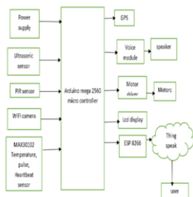
Fig 11: Block Diagram of proposed robot
