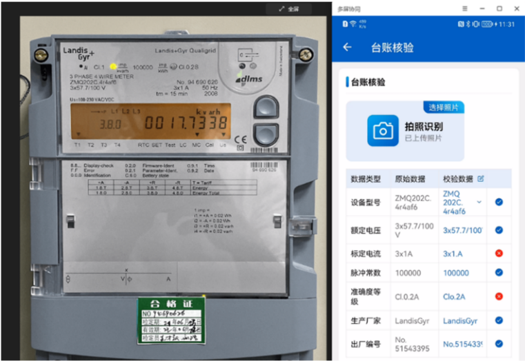
Figure 5. Verification results of the intelligent electric meter
