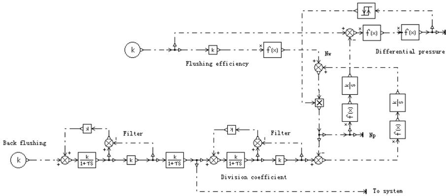
Figure 3. Back flushing simulation model
