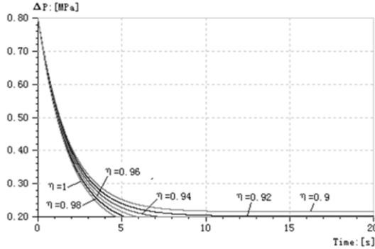
Figure 4. Effect of back flushing efficiency and results
