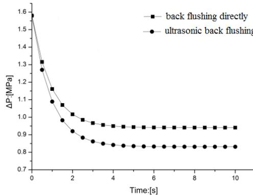
**Figure 6.** Experimental curves of back flushing directly and ultrasonic back flushing
