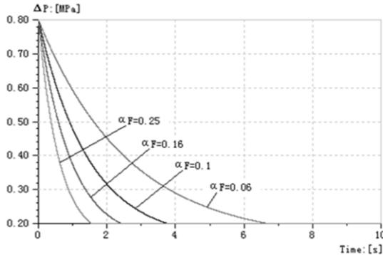
Figure 5. Effect of division coefficient and back flushing results
