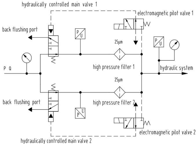
Figure 1. Principle of high pressure back flushing filter station
