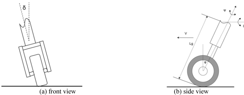
Figure 1. View of nose landing gear structure
